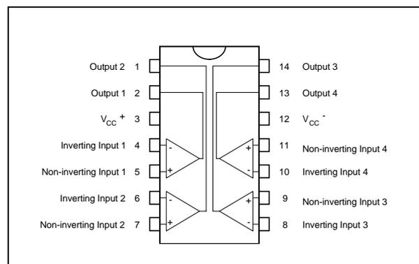
**SCHEMATIC DIAGRAM** (for 1/4 TS3V339)
